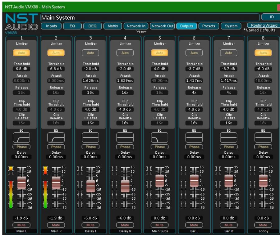
Outputs 1 & 2 are limiting in the above example and the heavy gain reduction can be seen in the metering (in addition to the level meters being at the end-stops in red!).
